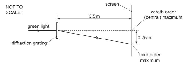
What is the distance between two adjacent slits in the diffraction grating?
