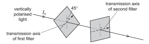
What is the intensity of the beam of light after transmission through the second filter?
