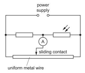
The light-dependent resistor (LDR) is then covered and the ammeter gives a non-zero reading.
